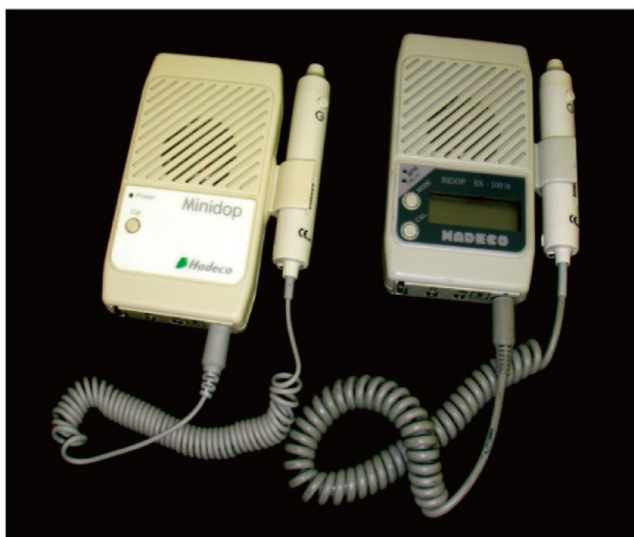
FIGURE 4 | Doppler auscultator: Only an auscultator (left) and one with a blood flow direction-detecting function (right) are available.
